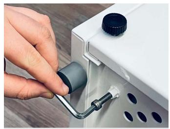
1 Loosen the four clamping screws on the bottom of the device with an Allen key. Screw out the screws by approx. 35 mm.
