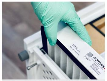
Remove the pre-filter from the housing. Then remove the activated carbon filter/gas filter and the HEPA H14 filter.
